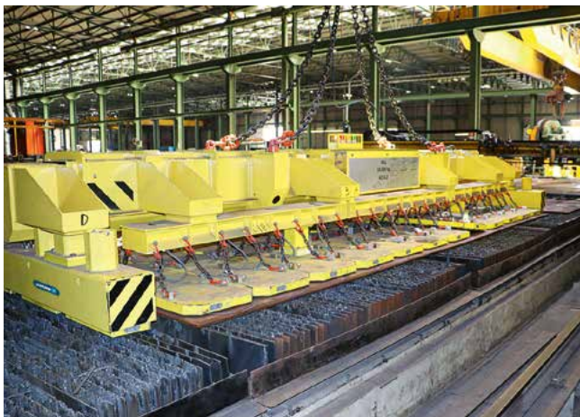
Hybrid traverse, hydraulically movable for loading and unloading of cutting systems up to 16 m
