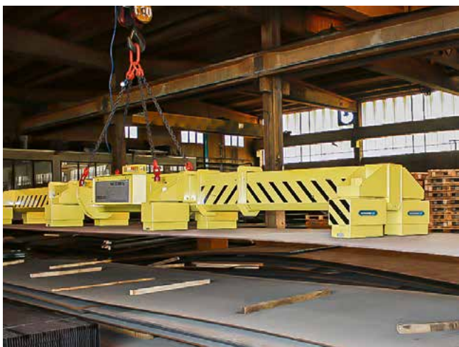
Magnetic traverse with extended hydraulic arms for loading of cutting systems
