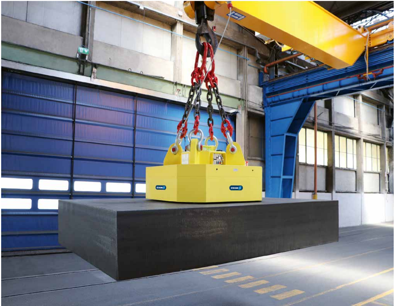
SEP Special for handling slabs up to 40 tons.
