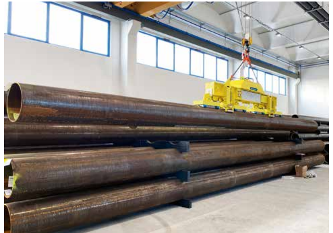
Handling of thin-walled long pipes
