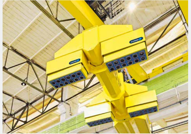
The magnetic pole packages were individually adapted to the application. With them, thin metal sheets from 5 mm can be handled.
