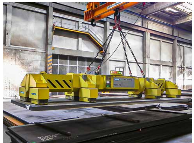
Magnetic traverse with retracted hydraulic arms for the transportation/ handling of thick sheet metal
