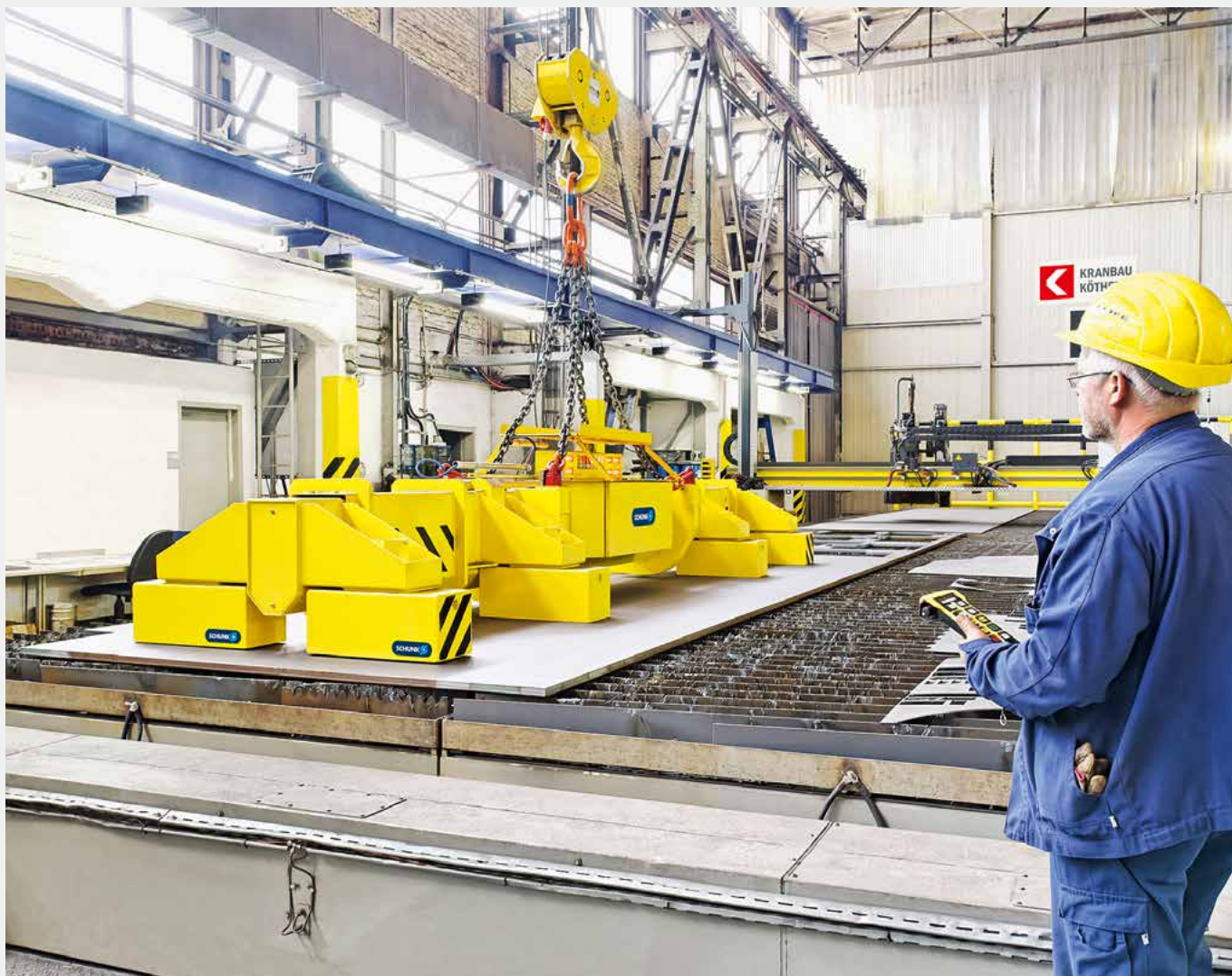
The separation of the sheets and the subsequent loading of the plasma cutting system were significantly simplified with the modular magnetic traverse.
